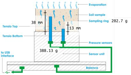
Evaporation experiment to determine K
