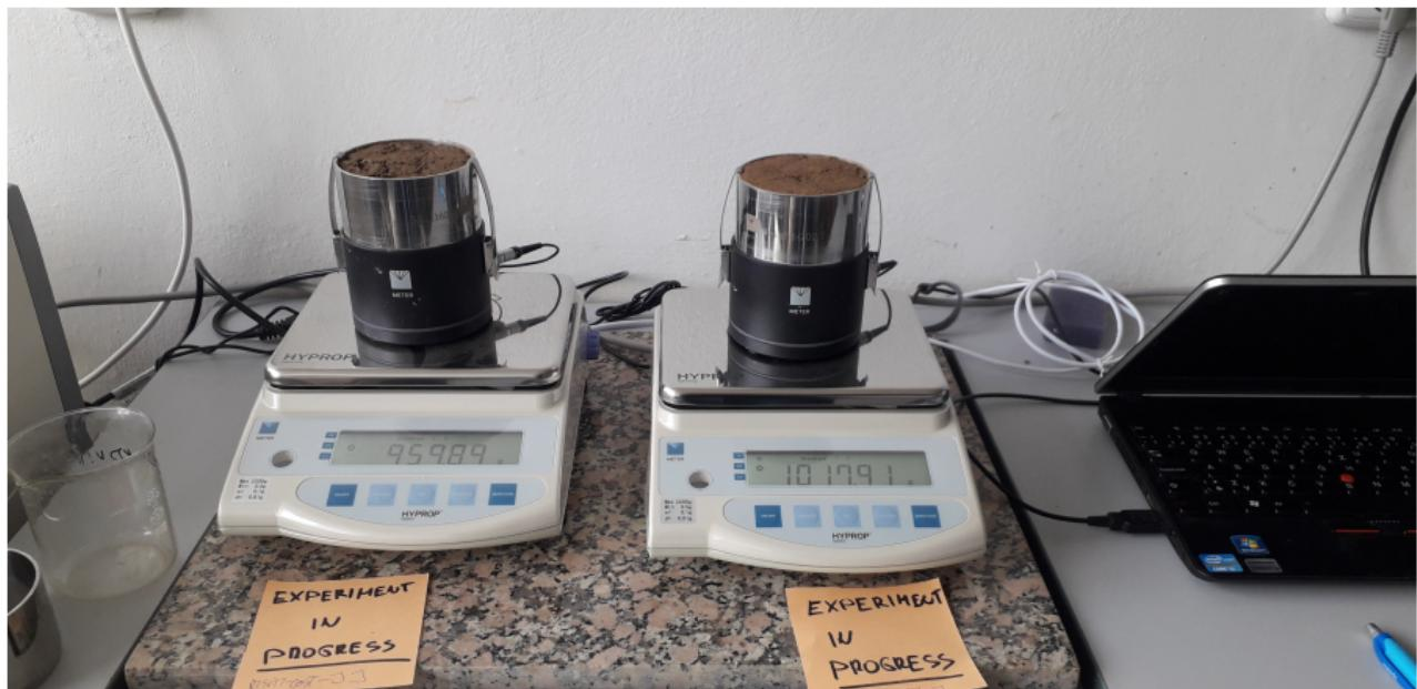
*Evaporation experiment to determine K*
