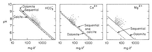
Figure 7.13 Chemical data from the Manitoban carbonate-rock aquifer plotted on diagrams showing equilibrium conditions at 5°C for open-system dissolution of calcite and dolomite and sequential dissolution of these two minerals (calcite before dolomite, which causes dolomite solubility to be depressed as a result of the common-ion effect). (After Cherry, 1972.)
