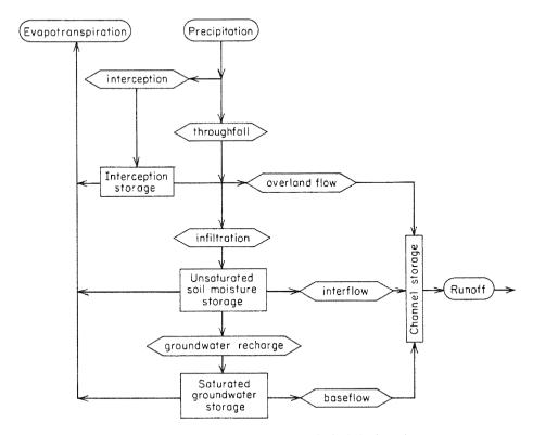
Figure 1.2 Systems representation of the hydrologic cycle.
