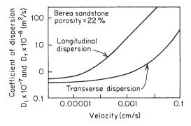
Figure 9.6 Coefficients of longitudinal and transverse dispersion for transport in a homogeneous sandstone at various flow rates (after Crane and Gardner, 1961).
