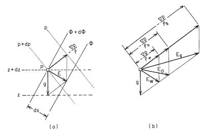
Figure 11.3 (a) Components of the impelling force *E* acting on a unit mass of water at a point *P* in a steady-state groundwater flow system; (b) impelling forces on water, oil, and gas in a three-phase steady-state flow system (after Hubbert, 1954).
