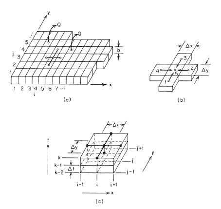
Figure 8.26 Discretization of a two-dimensional, horizontal, confined aquifer.
