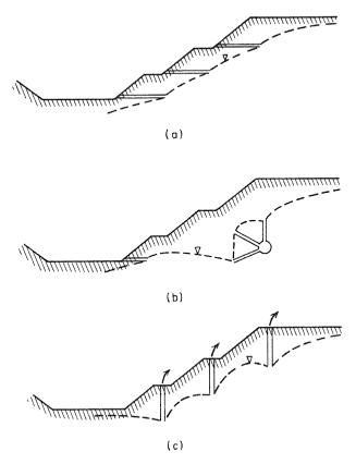
Figure 10.17 Dewatering excavations by (a) horizontal drains; (b) drainage gallery with radial drain holes; (c) three-stage wellpoint system.
