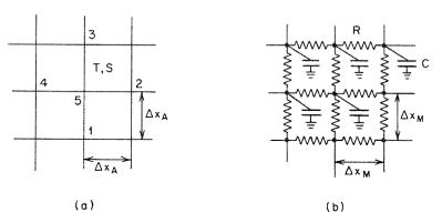
Figure 8.29 Small homogeneous portion of discretized aquifer and analogous resistor-capacitor network (after Prickett, 1975).
