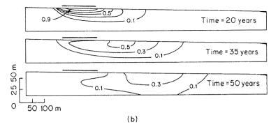
**Figure 9.13** Migration of a reactive contaminant through a shallow groundwater flow system. (a) Concentration versus time relation for the contaminant source; (b) concentration distributions after 20, 35, and 50 years. Porosity 0.3; hydraulic conductivity 0.5 m/day;  $\alpha_t = 10 \text{ m}$ ;  $\alpha_r = 0.5 \text{ m}$ ; concentration contours at  $C/C_0 = 0.9$ , 0.7, 0.5, 0.3, and 0.1 (after Pickens and Lennox, 1976).
