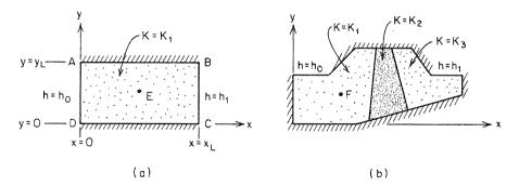
Figure 2.25 Two steady-state boundary-value problems in the xy plane.
