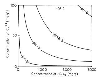
Figure 7.16 Solubility of calcite in water at 10°C expressed as a function of pH,  $Ca^{2+}$ , and  $HCO_3^-$ . Solubility lines computed from the relation  $K_{eq} = (Ca^{2+})(HCO_3^-)/(H^+)$ .
