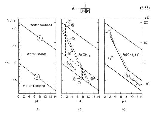
Figure 3.10 pE-pH diagrams, 25°C and 1 bar. (a) Stability field for water; (b) construction lines for the Fe-H<sub>2</sub>O system (see the text for equations representing number-designated lines); (c) completed diagram showing stability fields for major dissolved species and solid phases.
