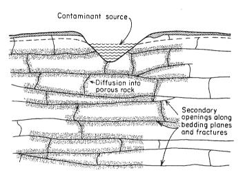
Figure 9.16 Schematic representation of contaminant migration from a surface source through fractured porous limestone.
