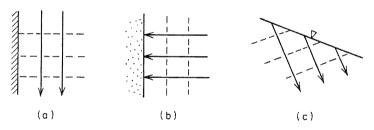
Figure 5.1 Groundwater flow in the vicinity of (a) an impermeable boundary, (b) a constant-head boundary, and (c) a water-table boundary.
