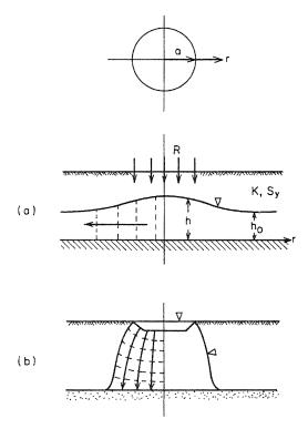
Figure 8.33 Growth of a groundwater mound beneath a circular recharge
