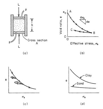
Figure 2.19 (a) Laboratory loading cell for the determination of soil compressibility; (b), (c), and (d) schematic curves of void ratio versus effective stress.
