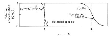
Figure 9.11 Advance of adsorbed and nonadsorbed solutes through a column of porous materials. Partitioning of adsorbed species is described by  $K_d$ . Relative velocity =  $1/[1 + (\rho_b/n)K_d]$ . Solute inputs are at concentration  $C_0$  at t > 0.
