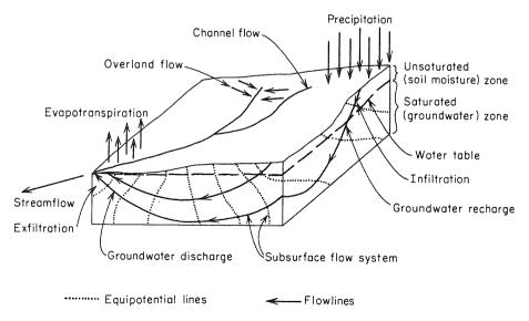
Figure 1.1 Schematic representation of the hydrologic cycle.
