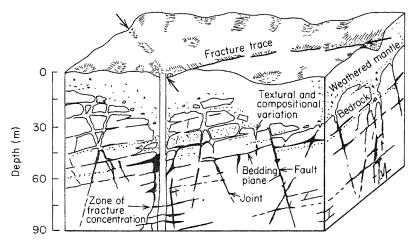
Figure 4.8 Occurrence of permeability zones in fractured carbonate rock.
