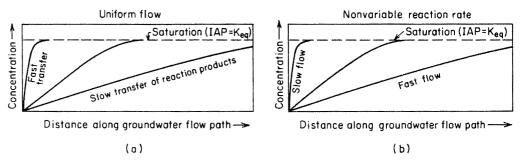
Figure 7.17 Schematic diagram showing the influence of (a) effective reaction rate and (b) flow rate on the distance along the flow path for saturation to be attained.
