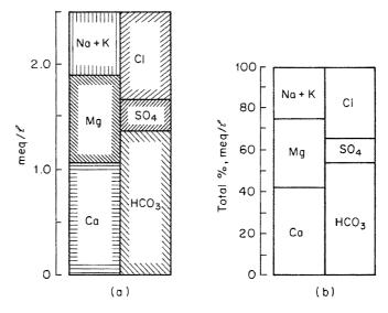
Figure 7.3 Chemical analyses of groundwater represented by bar graphs:
