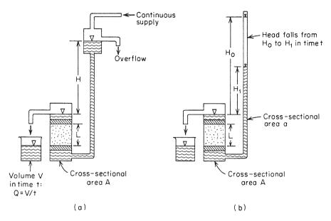
Figure 8.18 (a) Constant-head permeameter; (b) falling-head permeameter (after Todd, 1959).
