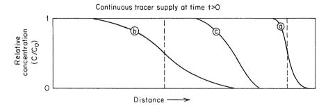
Figure 9.14 Advance of reactive and nonreactive contaminants through a column. (a) Dispersed front of nonretarded solute; (b) front of solute that undergoes equilibrium partitioning between liquid and solids; (c) front of solute that undergoes slower rate of transfer to the solids.
