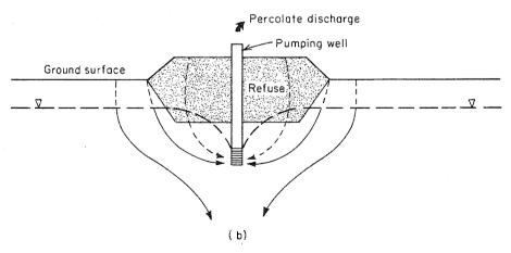
Figure 9.26 Control of leachate in a sanitary landfill by (a) tile drain or ditch and (b) pumped well (after Hughes et al., 1971).
