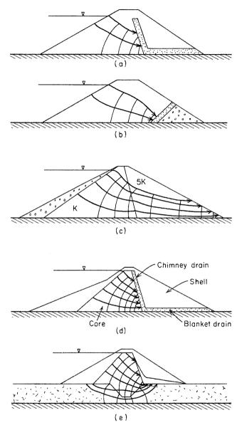
Figure 10.14 Design features for earth and rockfill dams (after Cedergren, 1967).
