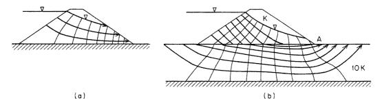
Figure 10.12 Flow nets for a homogeneous, isotropic earth dam on (a) impermeable foundation and (b) permeable foundation.
