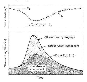
Figure 6.20 Streamflow hydrograph separation by the hydrochemical method.
