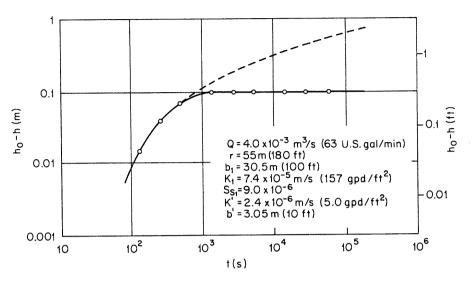
Figure 8.10 Calculated curve of  $h_0 - h$  versus t for a leaky aquifer, based on Hantush-Jacob theory.
