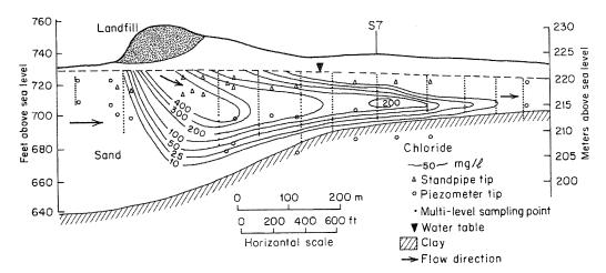
Figure 9.25 Plume of leachate migrating from a sanitary landfill on a sandy aquifer; contaminated zone is represented by contours of Cl-concentration in groundwater.
