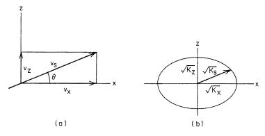
Figure 2.10 (a) Specific discharge  $v_s$  in an arbitrary direction of flow. (b) Hydraulic conductivity ellipse.
