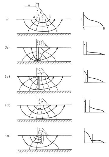
Figure 10.11 Uplift pressure profiles and flow nets for various grout curtain and drainage configurations.
