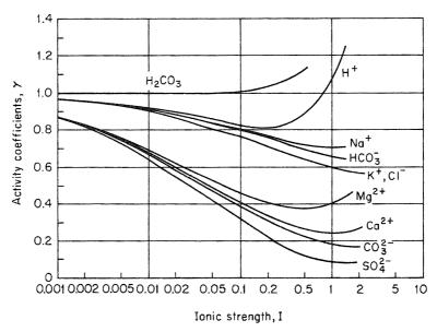
Figure 3.3 Activity coefficient versus ionic strength relations for common ionic constituents in groundwater.
