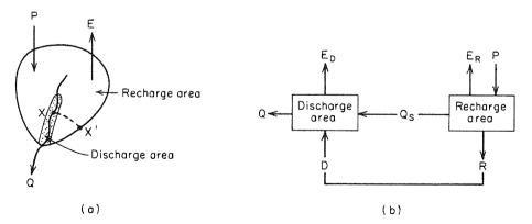
Figure 6.9 Steady-state hydrologic budget in a small watershed.
