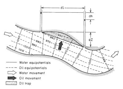
Figure 11.4 Vertical section through a plunging nose showing a hydrodynamically controlled oil trap (after Hubbert, 1954).
