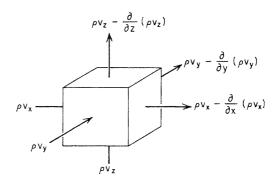
Figure 2.24 Elemental control volume for flow through porous media.
