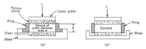
Figure 8.19 (a) Fixed-ring consolidometer; (b) floating-ring consolidometer (after Lambe, 1951).
