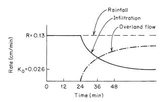
Figure 6.14 Time-dependent rates of infiltration and overland flow for the case shown in Figure 6.13 (after Freeze, 1974).
