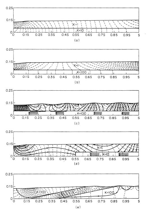
Figure 6.4 Effect of geology on regional groundwater flow patterns (after Freeze and Witherspoon, 1967).
