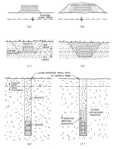
Figure 9.29 Schematic diagrams illustrating methods of low-level radioactive waste storage or disposal in shallow-water-table areas.
