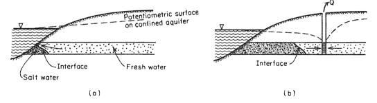
Figure 8.38 (a) Saltwater-freshwater interface in a confined coastal aquifer under conditions of steady-state seaward flow; (b) seawater intrusion due to pumping.
