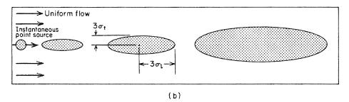
Figure 9.5 Spreading of a tracer in a two-dimensional uniform flow field in an isotropic sand. (a) Continuous tracer feed with step-function initial condition; (b) instantaneous point source.
