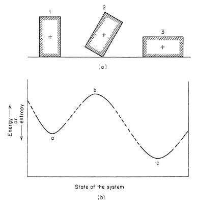
Figure 3.4 Concepts in mechanical and chemical equilibrium. (a) Metastable, unstable, and stable equilibrium in a mechanical system.
