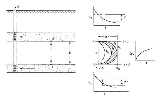
Figure 8.34 One-dimensional consolidation of an aquitard.
