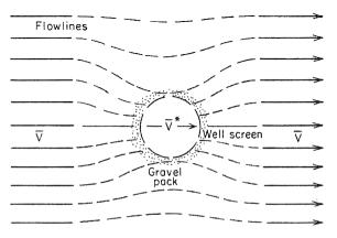
Figure 9.23 Distortion of flow pattern caused by the presence of the well screen and sand or gravel pack.
