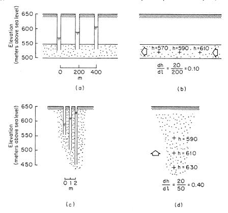
Figure 2.6 Determination of hydraulic gradients from piezometer installa-
