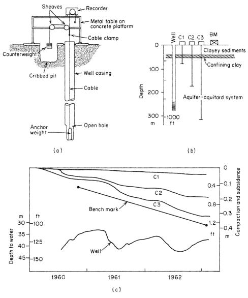
Figure 8.36 (a) Compaction-recorder installation; (b) compaction measurement site near Sunnyvale, California; (c) measured compactions, land subsidence, and hydraulic head variations at the Sunnyvale site, 1960–1962 (after Poland and Davis, 1969).
