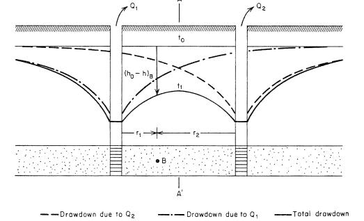
Figure 8.13 Drawdown in the potentiometric surface of a confined aquifer being pumped by two wells with  $Q_1 = Q_2$ .
