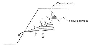
Figure 10.7 Slope stability analysis of a rock wedge (after Hoek and Bray, 1974).
