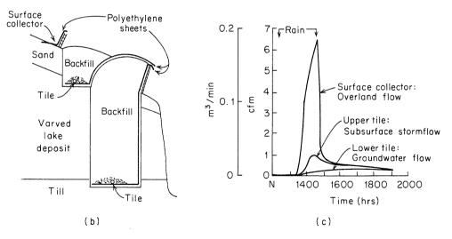
Figure 6.19 Sleepers River experimental watershed, Vermont. (a) Geologic cross section through the hillslope; (b) cross section of the interceptor trench; (c) combined hydrograph of flows during a sample storm (after Dunne and Black, 1970a).
