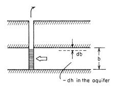
Figure 2.20 Aquifer compaction caused by groundwater pumping.
