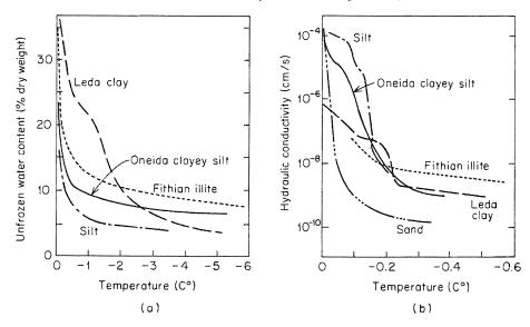
Figure 4.14 Effect of temperature on the hydraulic properties of several saturated soils. (a) Unfrozen water content versus temperature; (b) hydraulic conductivity versus temperature (after Burt and Williams, 1976).
