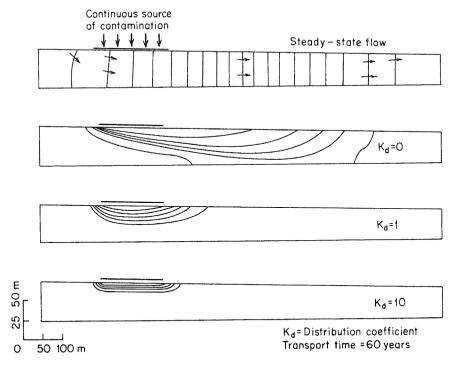
**Figure 9.12** Effect of the distribution coefficient on contaminant retardation during transport in a shallow groundwater flow system. Porosity 0.3; hydraulic conductivity 0.5 m/day;  $\alpha_l = 10$  m;  $\alpha_t = 0.5$  m; transport time 60 years; concentration contours at  $C/C_0 = 0.9$ , 0.7, 0.5, 0.3, and 0.1 (after Pickens and Lennox, 1976).
