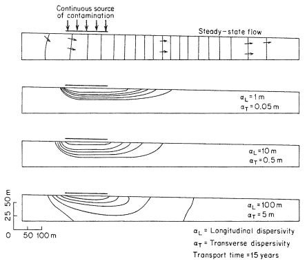
Figure 9.10 Dispersion of a contaminant during transport in a shallow groundwater flow system. Porosity 30%; hydraulic conductivity 0.5 m/day;  $\alpha_t/\alpha_t=20$ ; transport time 15 years; concentration contours at  $C/C_0=0.9,\,0.7,\,0.5,\,0.3$ , and 0.1 (after Pickens and Lennox, 1976).
