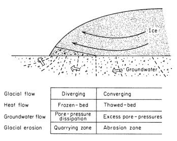
Figure 11.9 Interrelationships among glacial flow, heat flow, groundwater flow, and glacial erosion at the margin of a continental ice sheet (after Clayton and Moran, 1974).
