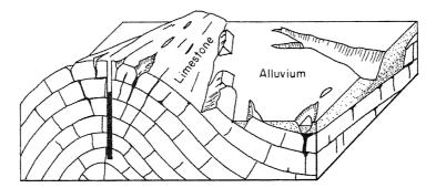
Figure 4.9 Occurrence of high-permeability zone in solution-enlarged fractures along the exposed crest of an anticline in carbonate rock (after Davis and De Wiest, 1966).
