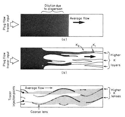
Figure 9.9 Comparison of advance of contaminant zones influenced by hydrodynamic dispersion. (a) Homogeneous granular medium; (b) fingering caused by layered beds and lenses; (c) spreading caused by irregular lenses.
