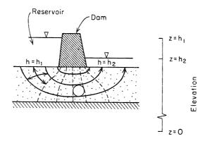
Figure 5.3 Seepage beneath a dam through homogeneous, isotropic foundation rocks.
