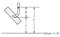
Figure 2.4 Hydraulic head h, pressure head  $\psi$ , and elevation head z for a laboratory manometer.
