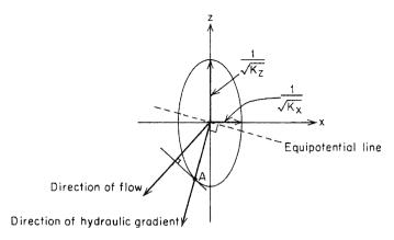
Figure 5.10 Determination of direction of flow in an anisotropic region with  $K_x/K_z = 5$ .
