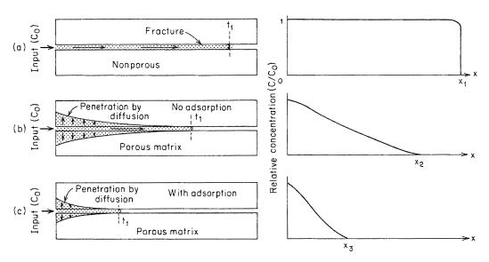
Figure 9.15 Effect of diffusion on contaminant migration in porous fractured medium. (a) Unidirectional hydraulic transport in a fracture in a nonporous medium; (b) unidirectional hydraulic transport with migration into matrix as a result of molecular diffusion; (c) unidirectional hydraulic transport with molecular diffusion and adsorption (profiles of relative concentration of reactive contaminant within fracture shown at time  $t_1$ ).
