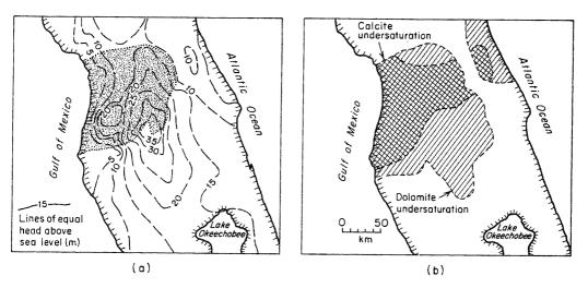
Figure 7.12 Regional limestone aquifer in south-central Florida. (a) Potentiometric surface and area of major recharge; (b) areas of undersaturation with respect to calcite and dolomite (after Hanshaw et al., 1971).
