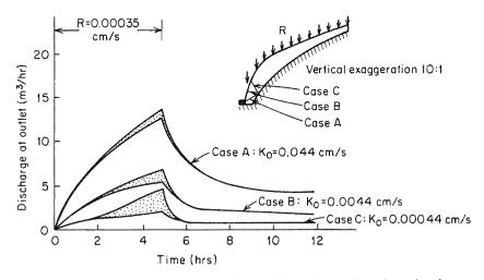
Figure 6.18 Numerically simulated streamflow hydrographs at the outlet of a hypothetical upstream source area in which the stream is fed by a convex hillslope having a shallow surface soil of high conductivity (after Freeze, 1974).
