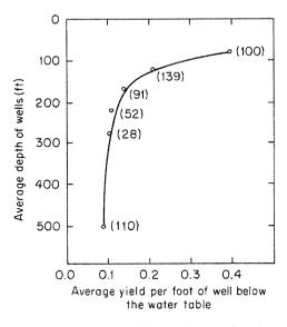
Figure 4.10 Decrease in well yields (gpm/ft of well below the water table) with depth in crystalline rocks of the Statesville area, North Carolina. Numbers near points indicate the number of wells used to obtain the average values that define the curve (after Legrand, 1954; Davis and De Wiest, 1966).
