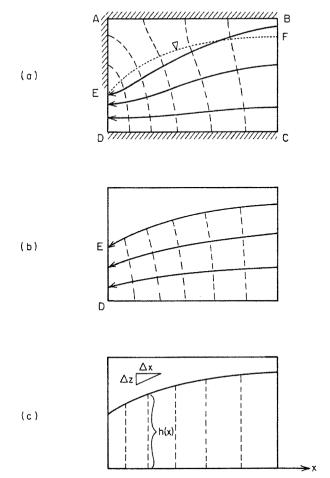
Figure 5.14 Development of a seepage face on a free-outflow boundary.
