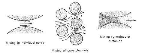
Figure 2.30 Processes of dispersion on a microscopic scale.
