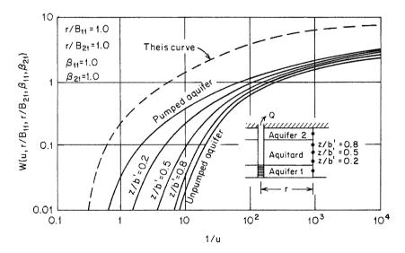
Figure 8.9 Theoretical curves of  $W(u, r/B_{11}, r/B_{21}, \beta_{11}, \beta_{21})$  versus 1/u for a leaky two-aquifer system (after Neuman and Witherspoon, 1969a).
