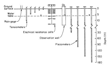
Figure 6.15 Field instrumentation for the investigation of groundwater recharge processes (after Freeze and Banner, 1970).
