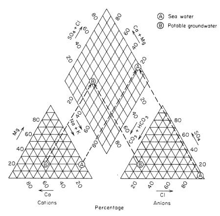
Figure 7.6 Chemical analyses of water represented as percentages of total equivalents per liter on the diagram developed by Hill (1940) and Piper (1944).
