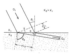
Figure 5.4 Refraction of flowlines at a geologic boundary.
