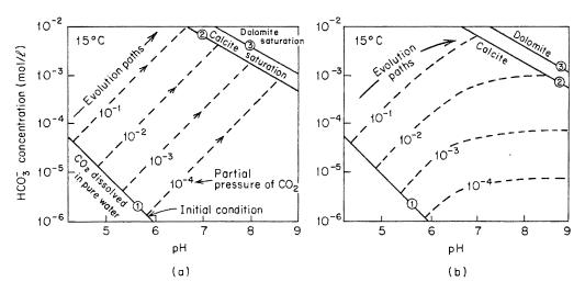
Figure 7.11 Chemical evolution paths for water dissolving calcite at 15°C.
