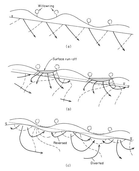
Figure 6.23 Depression-focused groundwater recharge in hummocky terrain (after Meyboom, 1966b).
