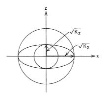
Figure 5.7 Hydraulic conductivity ellipse for an anisotropic medium with  $K_x/K_z = 5$ . The circles represent two possible isotropic transformations.
