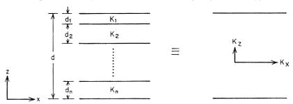
Figure 2.9 Relation between layered heterogeneity and anisotropy.
