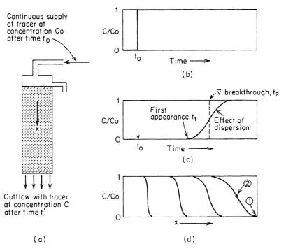
Figure 9.1 Longitudinal dispersion of a tracer passing through a column of porous medium. (a) Column with steady flow and continuous supply of tracer after time  $t_0$ ; (b) step-function-type tracer input relation; (c) relative tracer concentration in outflow from column (dashed line indicates plug flow condition and solid line illustrates effect of mechanical dispersion and molecular diffusion); (d) concentration profile in the column at various times.
