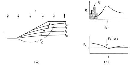
Figure 10.6 (a) Transient position of the water table during rainfall on a slope; (b) pore pressure at point C during and following a rainfall period; (c) factor of safety as a function of time during and following a rainfall period.
