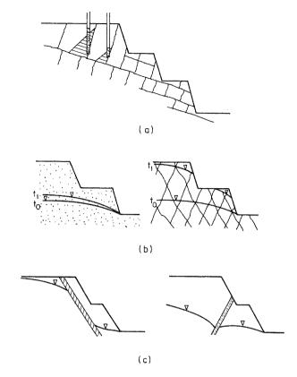
Figure 10.8 Some aspects of groundwater flow in rock slopes. (a) Possible large differences in fluid pressures in adjacent rock joints; (b) comparison of transient water-table fluctuations in porous soil slopes and low-porosity rock slopes; (c) fault as a low-permeability groundwater barrier and as a high-permeability subsurface drain (after Patton and Deere, 1971).
