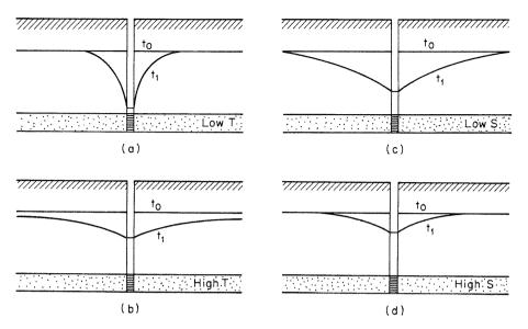
Figure 8.6 Comparison of drawdown cones at a given time for aquifers of
