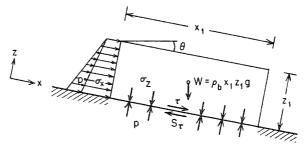
Figure 11.1 Stress equilibrium on a thrust block at incipient movement down an inclined fault plane (after Hubbert and Rubey, 1959).
