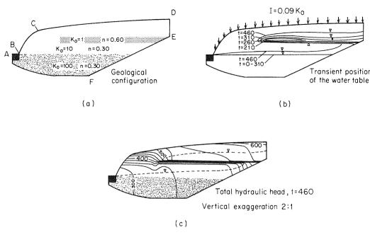
Figure 6.11 Formation of a perched water table (after Freeze, 1971a).
