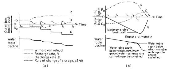
Figure 8.32 Schematic diagram of transient relationships between recharge rates, discharge rates, and withdrawal rates (after Freeze, 1971a).
