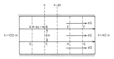
Figure 5.2 Quantitative flow net for a very simple flow system.
