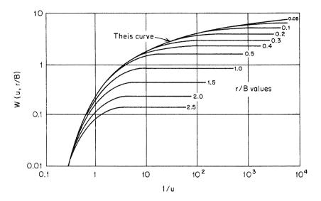
Figure 8.8 Theoretical curves of W(u, r/B) versus 1/u for a leaky aquifer (after Walton, 1960).
