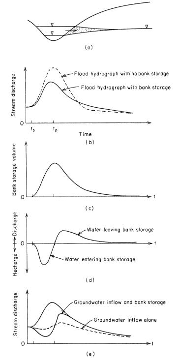
Figure 6.22 Flood-wave modification due to bank-storage effects.
