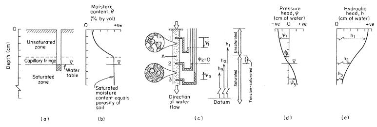
Figure 2.12 Groundwater conditions near the ground surface. (a) Saturated and unsaturated zones; (b) profile of moisture content versus depth; (c) pressure-head and hydraulic-head relationships; insets: water retention under pressure heads less than (top) and greater than (bottom) atmospheric; (d) profile of pressure head versus depth; (e) profile of hydraulic head versus depth.
