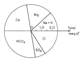
Figure 7.4 Chemical analysis of groundwater represented by a circular diagram. The radial axis is proportional to the total milliequivalents.
