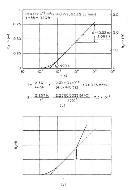
Figure 8.24 (a) Determination of T and S from  $h_0 - h$  versus t data using the semilog method; (b) semilog plot in the vicinity of an impermeable boundary.
