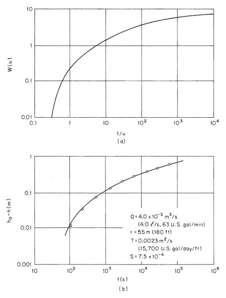
Figure 8.5 (a) Theoretical curve of W(u) versus 1/u. (b) Calculated curve of  $h_0 - h$  versus t.
