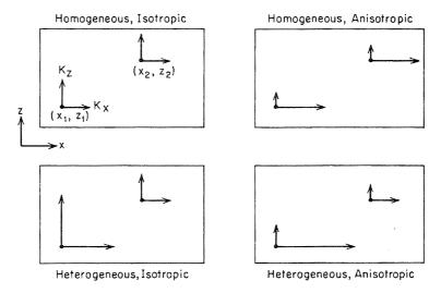
Figure 2.8 Four possible combinations of heterogeneity and anisotropy.
