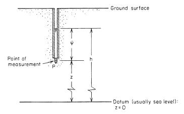
Figure 2.5 Hydraulic head h, pressure head  $\psi$ , and elevation head z for a field piezometer.
