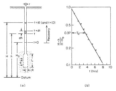
Figure 8.20 Hyorslev piezometer test. (a) Geometry; (b) method of analysis.
