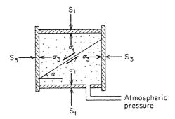
Figure 10.2 Schematic representation of laboratory setup for drained triaxial test.
