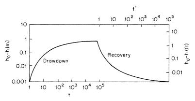
Figure 8.14 Schematic diagram of the recovery in hydraulic head in an aquifer after pumping is stopped.
