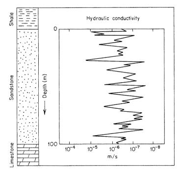
Figure 4.6 Schematic diagram of hydraulic conductivity versus depth relation for a thick, relatively homogeneous sandstone aguifer.
