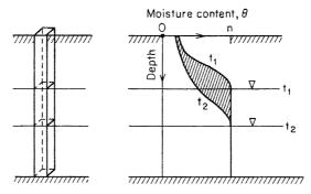
Figure 2.23 Concept of specific yield viewed in terms of the unsaturated moisture profiles above the water table.
