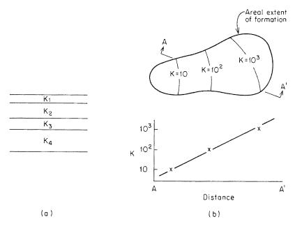
Figure 2.7 Layered heterogeneity and trending heterogeneity.
