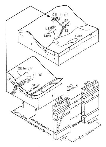
Figure 11.11 Schematic diagram showing the development of geochemical anomalies in an area where bedrock is overlain by a residual soil (after Bradshaw, 1975).
