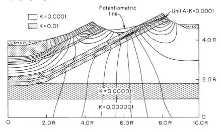
Figure 10.9 Hydrogeologic regime in thrusted sedimentary environment.
