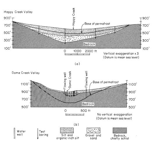
Figure 4.15 Hydrogeologic sections across two valleys in the Fairbanks mining district, Alaska. (a) Occurrence of sand and gravel aquifer below the base of permafrost; (b) sand and gravel deposit that is frozen in the permafrost zone. Flowing wells occur below the base of the permafrost (after Williams, 1970).
