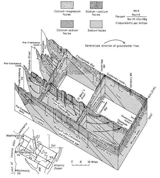
Figure 7.10 Fence diagram showing cation facies and generalized directions of groundwater flow in part of the northern Atlantic Coastal Plain (after Back, 1961).
