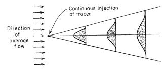
Figure 2.29 Schematic representation of the dilution process caused by mechanical dispersion in granular porous media.
