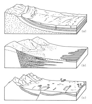
Figure 4.1 Influence of stratigraphy and structure on regional aquifer occurrence. (a) Gently dipping sandstone aquifers with outcrop area along mountain front; (b) interfingering sand and gravel aquifers extending from uplands in intermountain region; (c) faulted and folded aquifer in desert region. Surface water bodies reflect structural features (after Hamblin, 1976).
