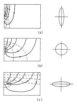
Figure 5.9 Flow nets for the flow problem of Figure 5.8(a) for  $\sqrt{K_x}/\sqrt{K_z}$  = (a) 1/4, (b) 1, (c) 4 (after Maasland, 1957).
