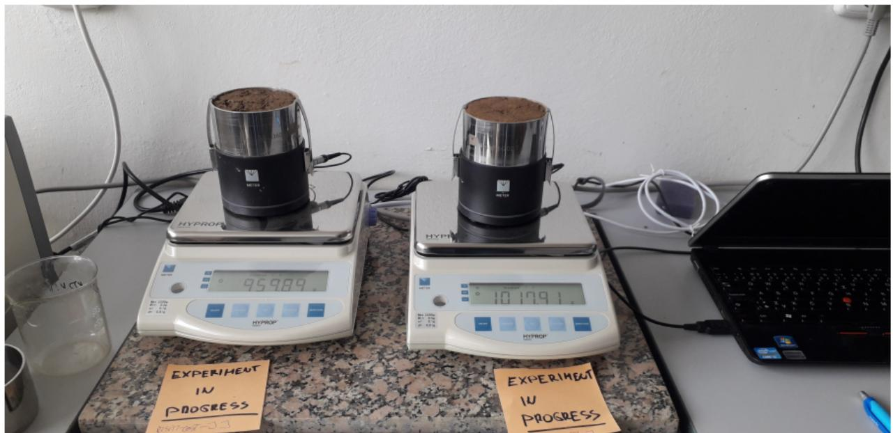
*Evaporation experiment to determine K*
